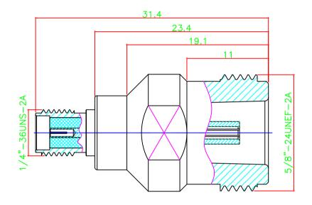
Note: Do Turn Male (Plug) Connector Nut (Shell) Only To Tighten
