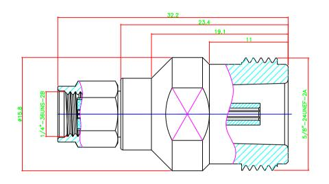
Note: Do Turn Male (Plug) Connector Nut (Shell) Only To Tighten
